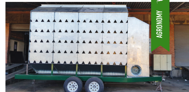
A mobile continual flow grain dryer called the Mobidry by Fangveiv – see ZiMunda Issue 6.
